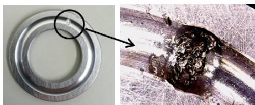
Fig.7 Flaking of Inner Race
