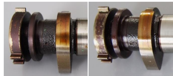
Figure 4. Effects of Reducing Additive on Camshaft Cleaning
