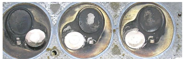
Removal of Carbon and Deposit in Combustion Chamber
