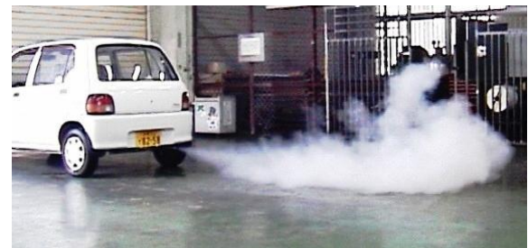
Figure 5. Emission of White Smoke
