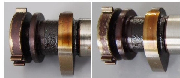
Figure 4. Effects of Reducing Additive on Camshaft Cleaning
